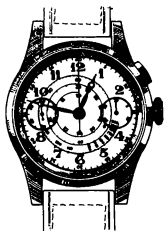
TACHYMETER CHRONOGRAPH. This dial is calibrated similar to the tachymeter already illustrated with the exception that the spiral in the centre indicates the miles per hour over a measured mile. Therefore one revolution of the seconds hand indicates 60 m.p.h., 2 revolutions 30 m.p.h. and 3 revolutions 20 m.p.h.
