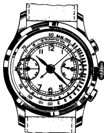
An example of chronograph dial calibrated to show the tachymeter and the telemeter combined.
